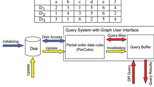
Figure 3: The proposed system based on the partial order data cube (ParCube) (this figure is best viewed in color)
