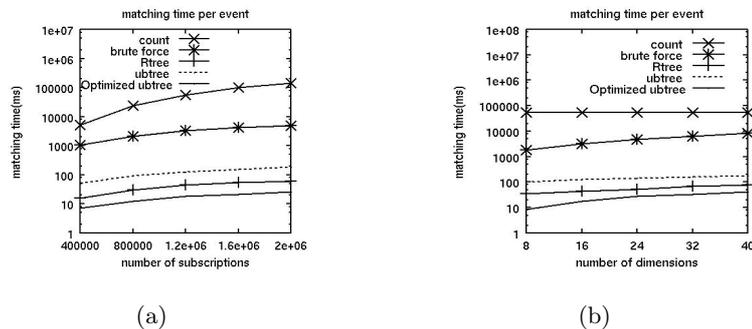
**Fig. 1.** Performance Examples of Event Filtering Based on Different Index Techniques
