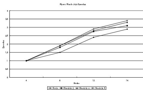
Figure 9. Speed Up versus the Number of processors: Rivers/Rivers
