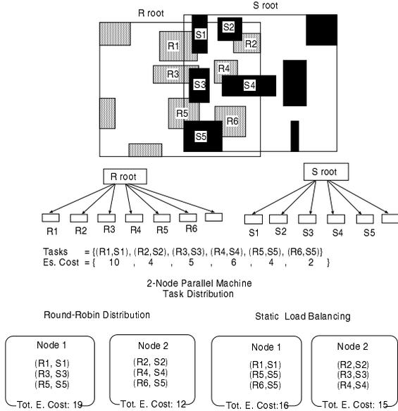
Figure 3. Filter Task Creation and Distribution in Parallel R-tree Join
