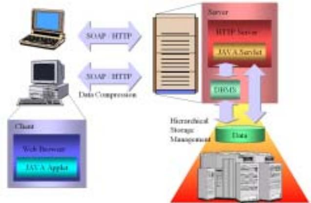
**Figure2:** Architecture of Data Integration System.
