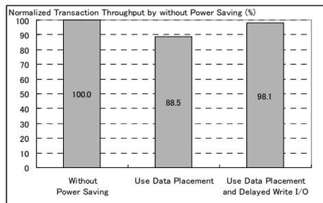
**Fig. 18: Transaction Throughput (Five Disk Drives for DBMS with Delayed Write I/O).**
