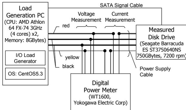
Fig. 1: Measurement Environment of Drive Disk Power Consumption.
