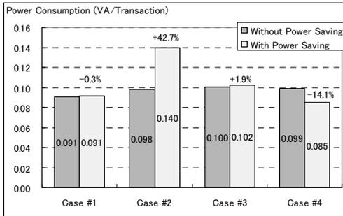
**Fig. 9: Power Consumption per Transaction (Measured Values; Two Disk Drives for DBMS).**
