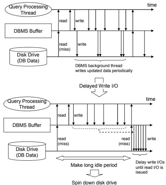
Fig. 6: Delayed Write I/O.
