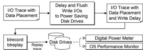
**Fig. 11: Simulation Method for Write Delay.**
