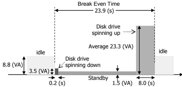
Fig. 3: Power Consumption of Standby Status and Break-Even Time.
