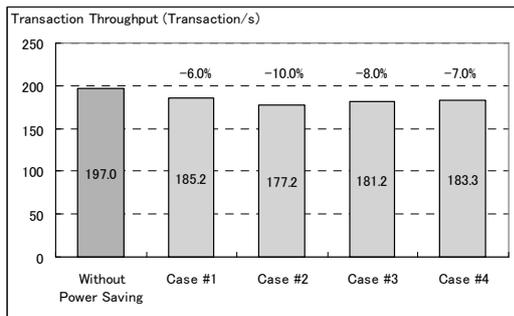
Fig. 14: Transaction Throughput (Two Disk Drives for DBMS with Delayed Write I/O).
