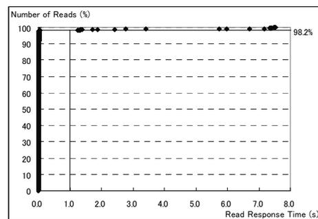
Fig. 15: Read response time and Number of Read I/Os (With Power Savings).
