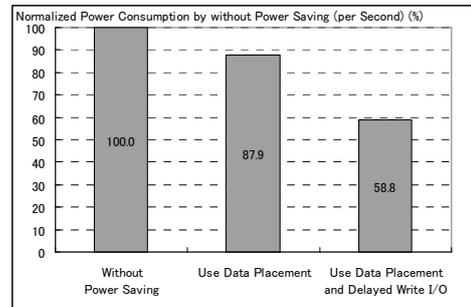
**Fig. 16: Power Consumption (Five Disk Drives for DBMS with Delayed Write I/O).**
