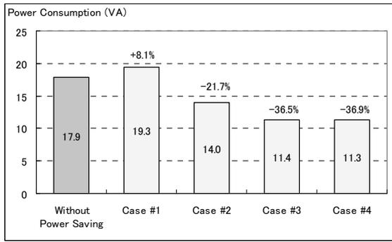
Fig. 12: Power Consumption (Two Disk Drives for DBMS with Delayed Write I/O).
