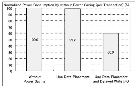
**Fig. 17: Power Comparison per Transaction (Five Disk Drives for DBMS with Delayed Write I/O).**
