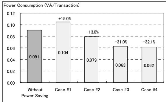
Fig. 13: Power Consumption per Transaction (Two Disk Drives for DBMS with Delayed Write I/O).
