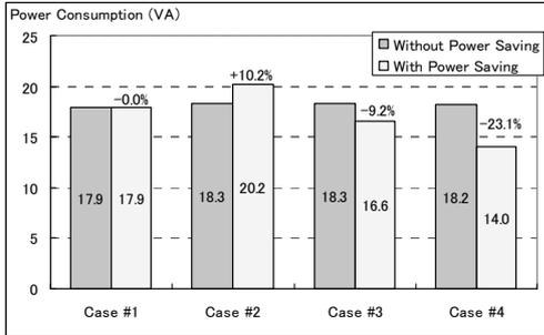
**Fig. 8: Power Consumption (Measured Values; Two Disk Drives for DBMS).**
