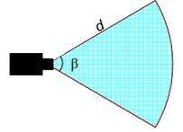
Fig. 1. A camera sensor with its FoV ( $\beta$ ) and DoF ( $d$ )
