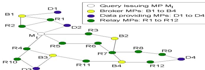
**Fig. 1.** Illustrative example of an instance of network topology
