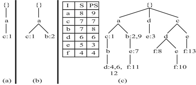
Fig. 5. Construction of GPF-Tree. (a) After scanning first transaction (b) After scanning second transaction and (c) After scanning entire database.
