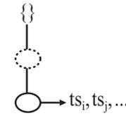
**Fig. 3.** Conceptual structure of prefix-tree in GPF-tree. Dotted ellipse represents ordinary node, while other ellipse represents tail-node of sorted transactions with timestamps  $ts_i, ts_j \in R$ .
