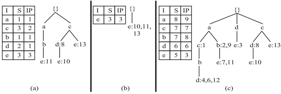
Fig. 6. Recursive mining of GPF-Tree. (a) Prefix-tree for 'f' (b) Conditional-tree for 'f' and (c) GPF-tree after removing the item 'f'.
