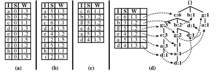
Fig. 2: Construction of WFIM-tree. (a) WFIM-list before scanning the database (b) WFIM-list after scanning the entire database (c) Final WFIM-list (d) Final WFIM-tree
