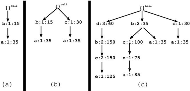
Fig. 2: Construction of SWFP-tree. (a) After scanning first transaction (b) After scanning second transaction and (c) After scanning the entire database
