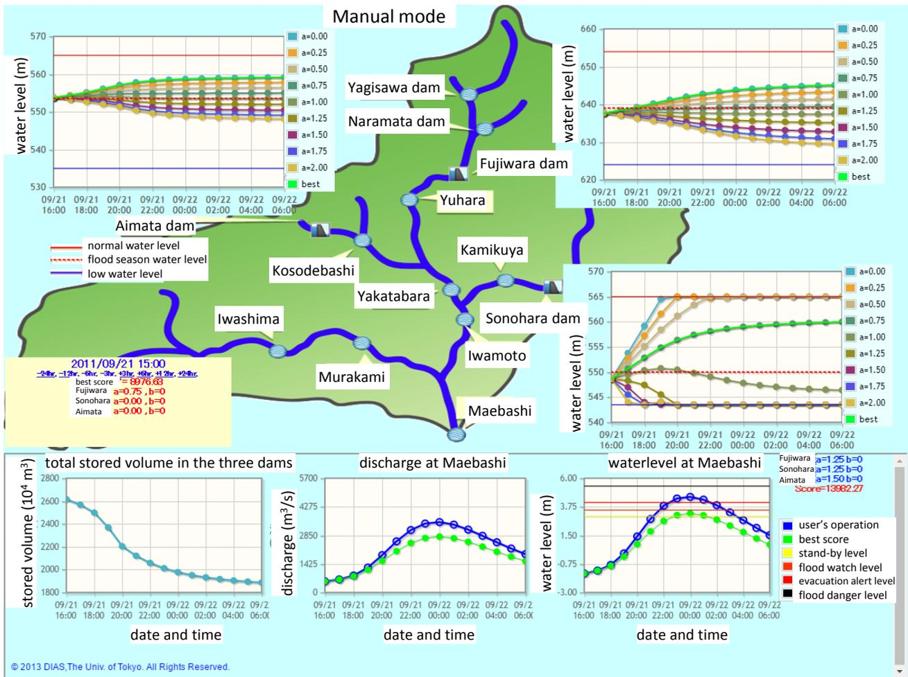
Fig. 6. Screenshot of the virtual reservoir simulator model. The results are linked to the DIAS data archive and users of the system can perform virtual simulations of the reservoirs interactively.
